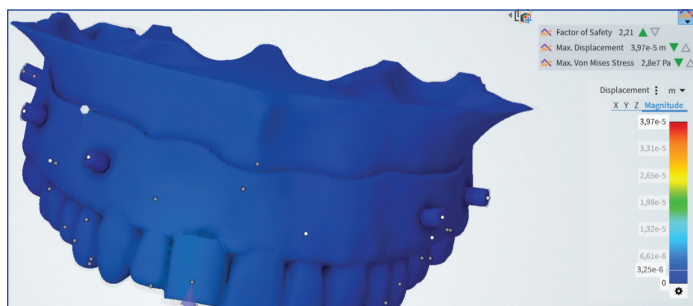
[Table/Fig-13]: FEA stress distribution of anchor pin-supported palatal surgical guide.
