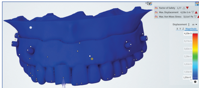
[Table/Fig-10]: FEA stress distribution of anchor pin-supported complete surgical guide.
