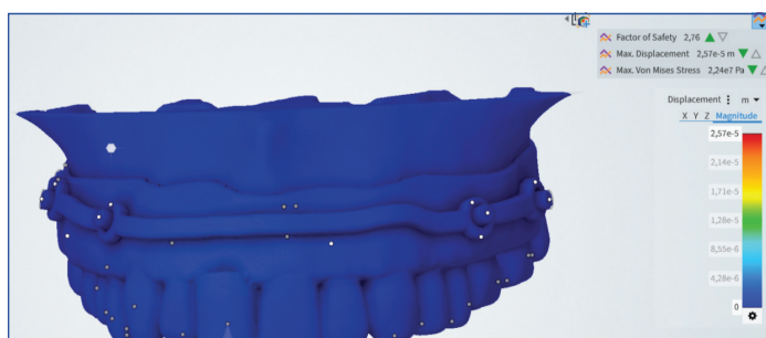
[Table/Fig-14]: FEA stress distribution of bend plate-supported palatal surgical guide.
