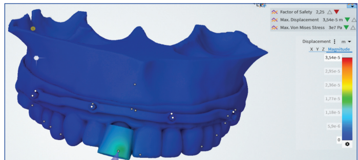
[Table/Fig-8]: FEA stress distribution of bend plate-supported pilot surgical guide.
